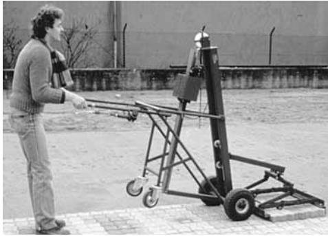
Figure 3. Non-motorized equipment used to set a small layer of pavers.
