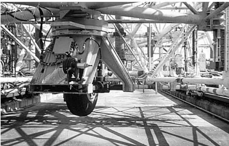
Figure 7. Test equipment for evaluation of the friction properties of concrete pavers at NASA's Aircraft Dynamics Landing Facility (ADLF) in Langley, Virginia
