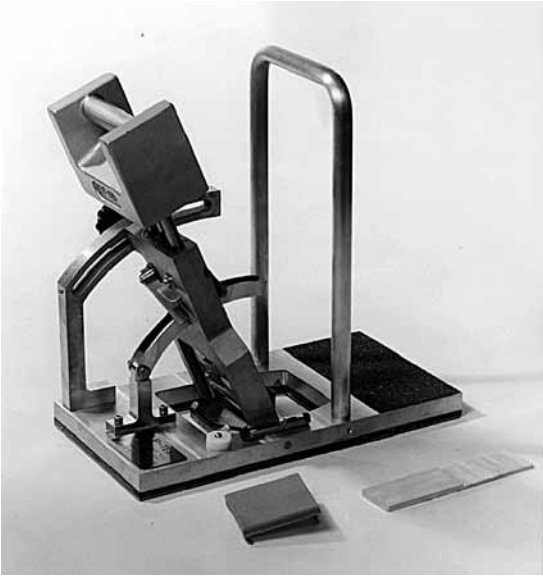
Figure 2. The NIST-Brungraber Mark II tester for slip resistance
