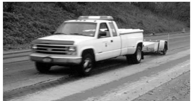
Figure 4. ASTM E 274 Test Equipment consists of a truck and trailer assembly. A tire within the trailer is towed at a given speed, locked, and skidded across water dispensed on the pavement in front of it.
