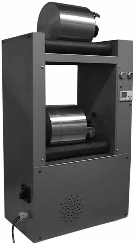
Figure 1. The Micro-Deval test apparatus. Photo courtesy of Geneq, Inc.
