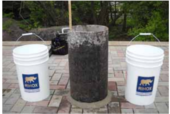
The permeability field test apparatus - steel casing shown above paver surface.
